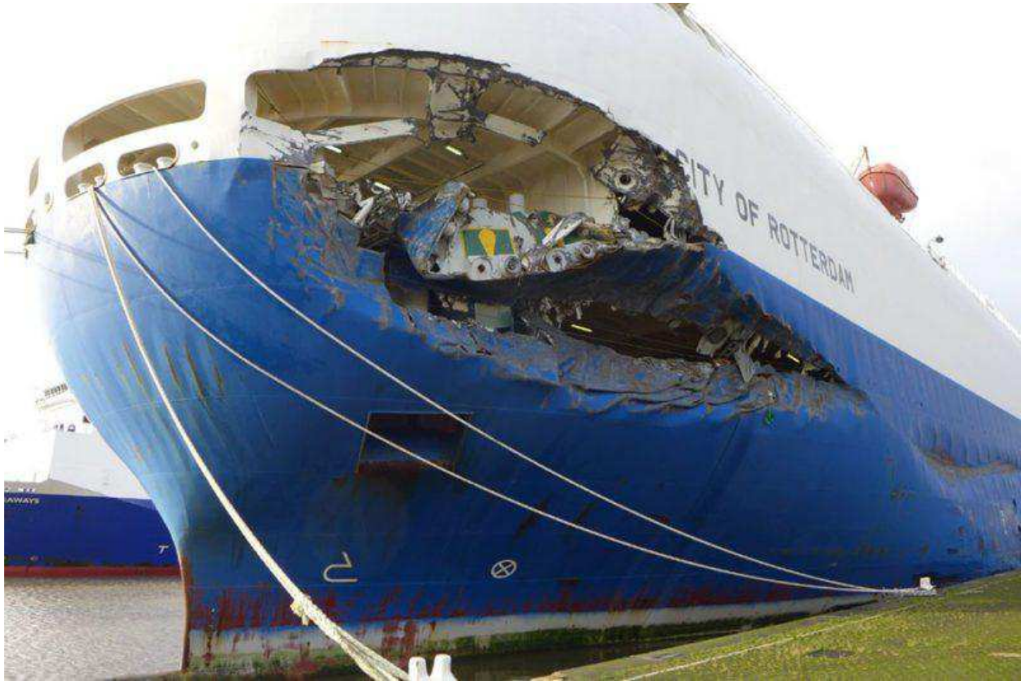
Damage to the City of Rotterdam after colliding with the Danish-flagged Primula Seaways on the River Humber on December, 3, 2015. Photo: MAIB
